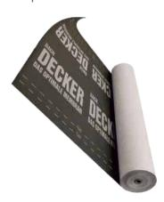
Diffusive membrane with a triple-layer design weighing approximately 135 g/m2. It is highly permeable to water vapour and very durable. Resistant to UV rays. This is an original product manufactured by molecular bonding of the layers using ultrasound. Ultrasound technology makes it possible to achieve a very strong membrane while maintaining strong diffusion properties.
