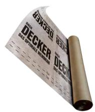
The DEKER REFLEX membrane with a reflecting layer of aluminium is an original product produced by the ultramodern ultrasound molecular bonding technology. This membrane makes it possible to actively regulate vapour transmission capacity and dry the insulation and wooden structures. Meanwhile, the reflecting surface of the aluminium coating means heat loss inside the house can be reduced.
